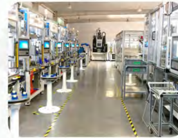
电动助力转向器（EPS）装配检测线 Electric power steering (EPS) assembling and testing line
