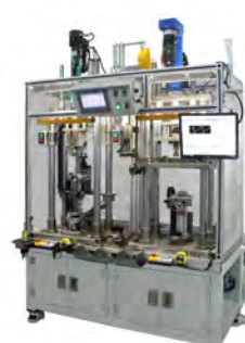
柱管总成与芯轴总成装配台 Pipe assembly and mandrel assembling
