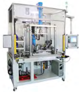
转向轴总成与壳蜗组件合成台 Steering axle and volute assembling
